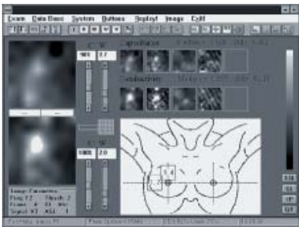
Figure 17 Screen display in the targeted mode. The region of interest (lesion, suspected lesion) is scanned, and independently recorded. Up to five sectors are saved, their locations corresponding to numbered positions on the anatomic sketch.
